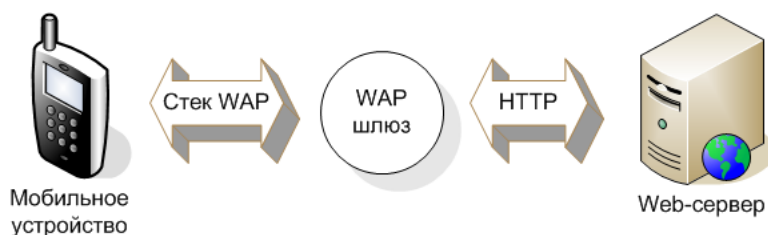
Figure 4 - Interaction of the mobile device with the Internet server.
